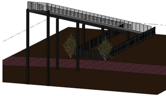
Figure 14: Rendered toboggan chute fence alternative
